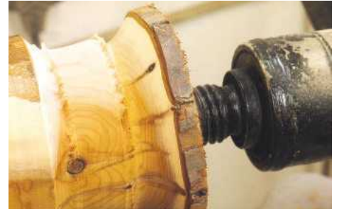
▲ Pic.2 Once it's mounted in the chuck turn down the underneath of the edge to a simple curve; keep the tailstock in as long as you can for added security
